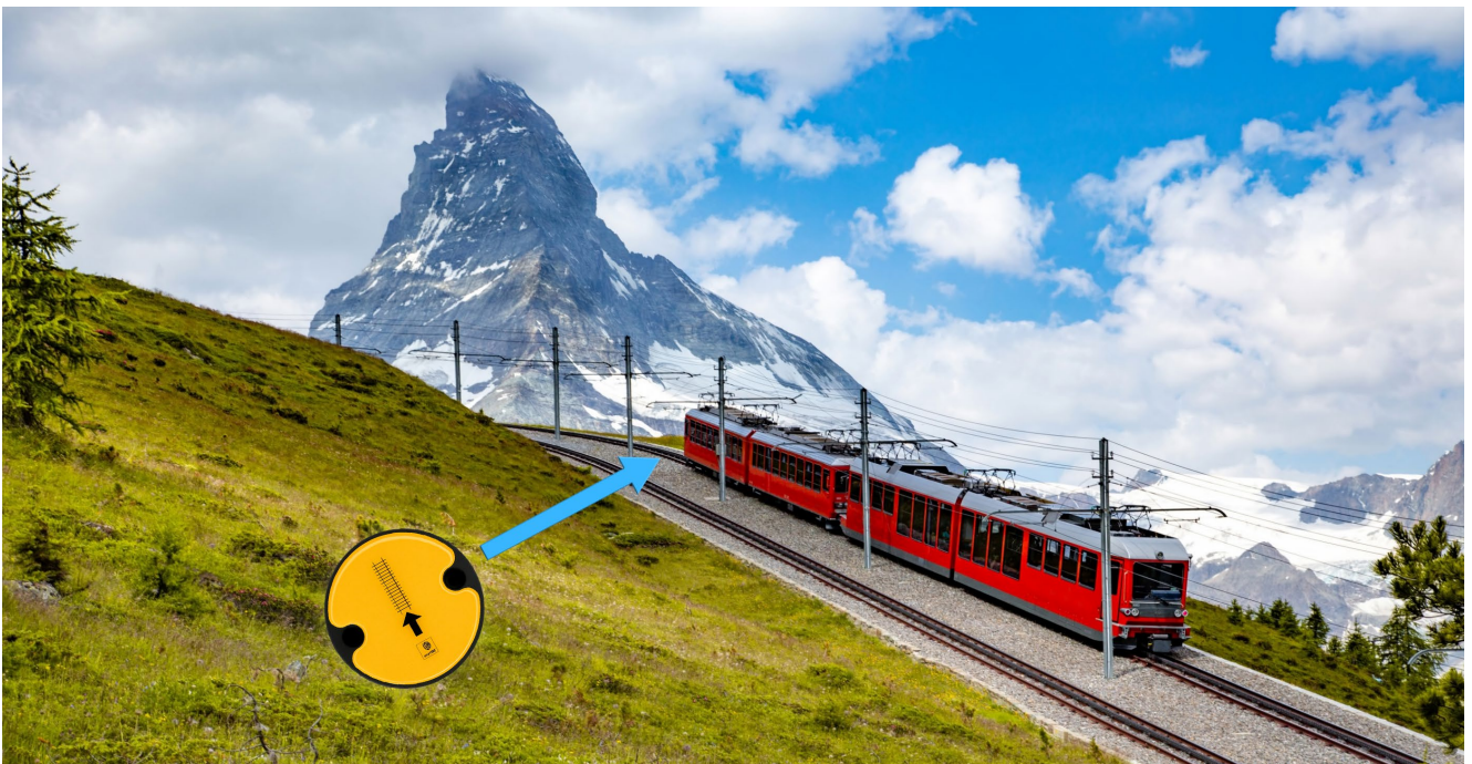
Winding railway line in the Alps; special railblock transponders from smart TEC are laid in the track bed.
